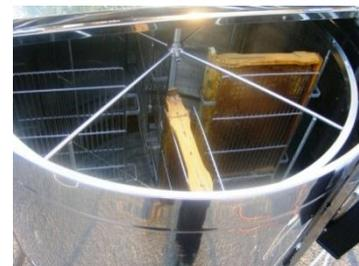
The option of changing direction twice instead of three times is also available. The method is included in the instructions for use of the regulating electronics. The extractor indicates the end of the program by giving a beeping sound.
