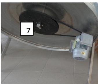
Check the V-pulley at the bottom of the unit for secure fastening on the axis. Adjust it using the screw on the V-pulley if necessary. Check V-pulleys for line run and the V-belt for tightness. If the V-belt is not on the pulley then place it.
